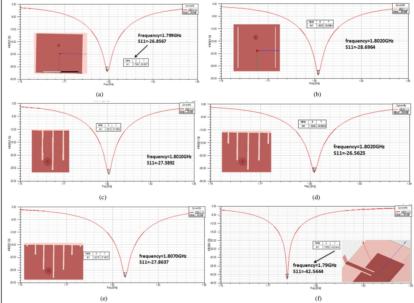
Figure 3. Return loss Vs Frequency for rectangular microstrip antenna (a. with slot coax feed, b. 2 slots with coax feed, c. 3 slots with coax feed, d. 5 slots with coax feed, e. 7 slots with coax feed, f. inset with microstrip feed)
