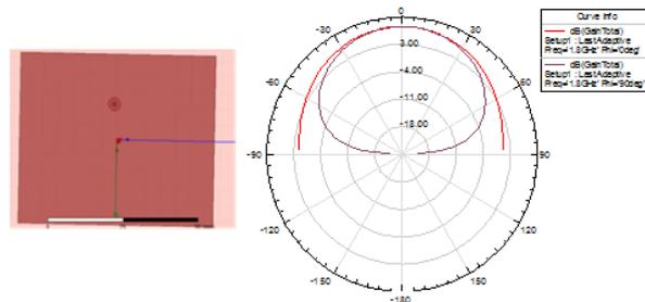
Figure 4. Radiation Pattern for rectangular microstrip antenna
